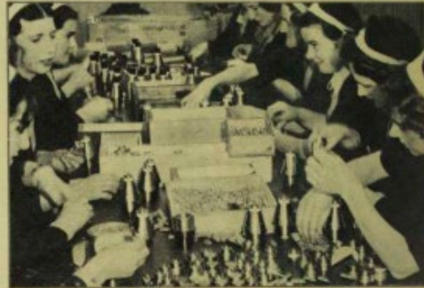
Finished Product Fuses being assembled in an Australian factory. They contain fulminate of mercury. Fulminate results from treatment of mercury with nitric acid, alcohol. Explosion of mercuric fulminate is so violent, rapid, that it has to be modified by mixture with other chemicals for use in munitions. Pure fulminate is so sensitive that tick of a finger-nail is sufficient to cause it to explode. Usually, it is handled only in small lots.
