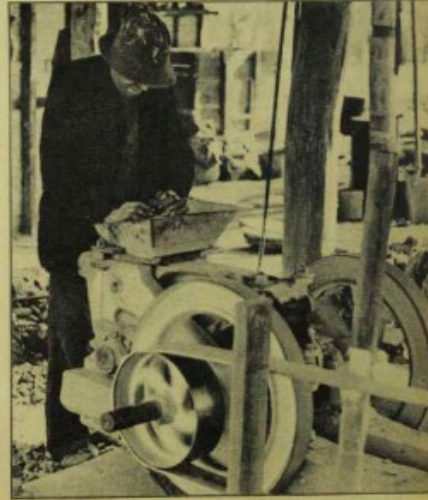
Crushing Cinnabar, brought from mine in large lumps, is broken up before treatment in retorts. Power crusher is used for this purpose. Cinnabar ranges in color from a dark brown to brilliant red.
