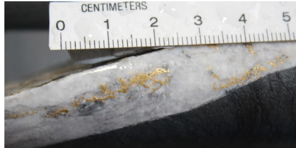
Photograph 54: Gold in quartz within carbonaceous siltstone, Pengelly Siltstone Member. In GEGM drill hole L068, depth 60.6 m, drilled from Stockwork 6A, Monkland Mine.
